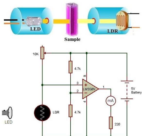
Fig. 1. Design and circuit of suggested device.
