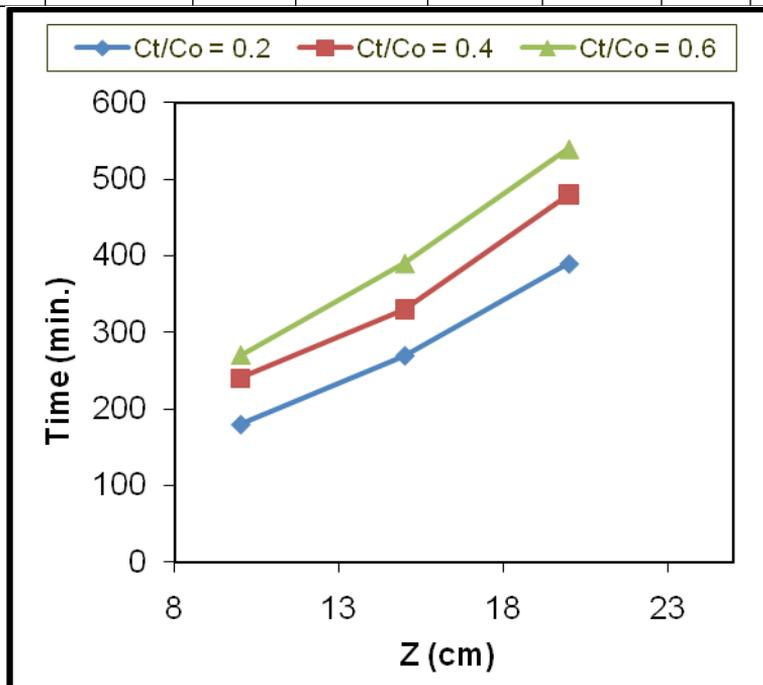
**Fig. 7. Isoremoval lines for 0.2,0.4,0.6 breakthrough for different bed height ( $C_o = 20\text{ mg l}^{-1}$ ,  $F = 1\text{ ml min}^{-1}$ )**
