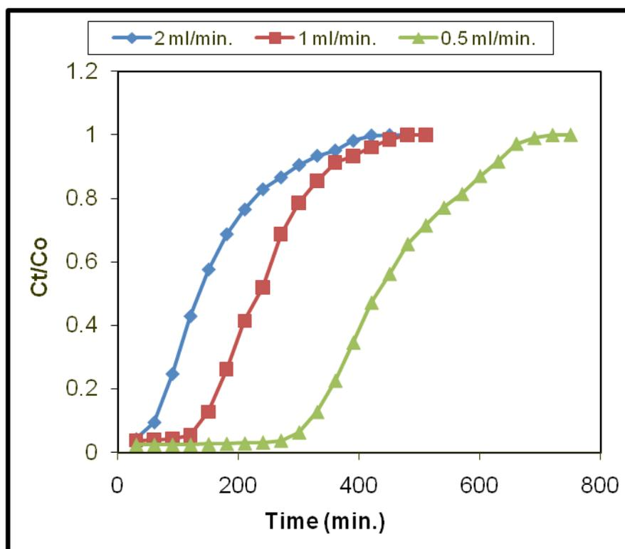
Fig. 2. Breakthrough curves of the effects of flow rates on biosorption of CR onto water hyacinth ( $F = 1 \text{ ml min}^{-1}$ ,  $C_o = 20 \text{ mg l}^{-1}$ )
