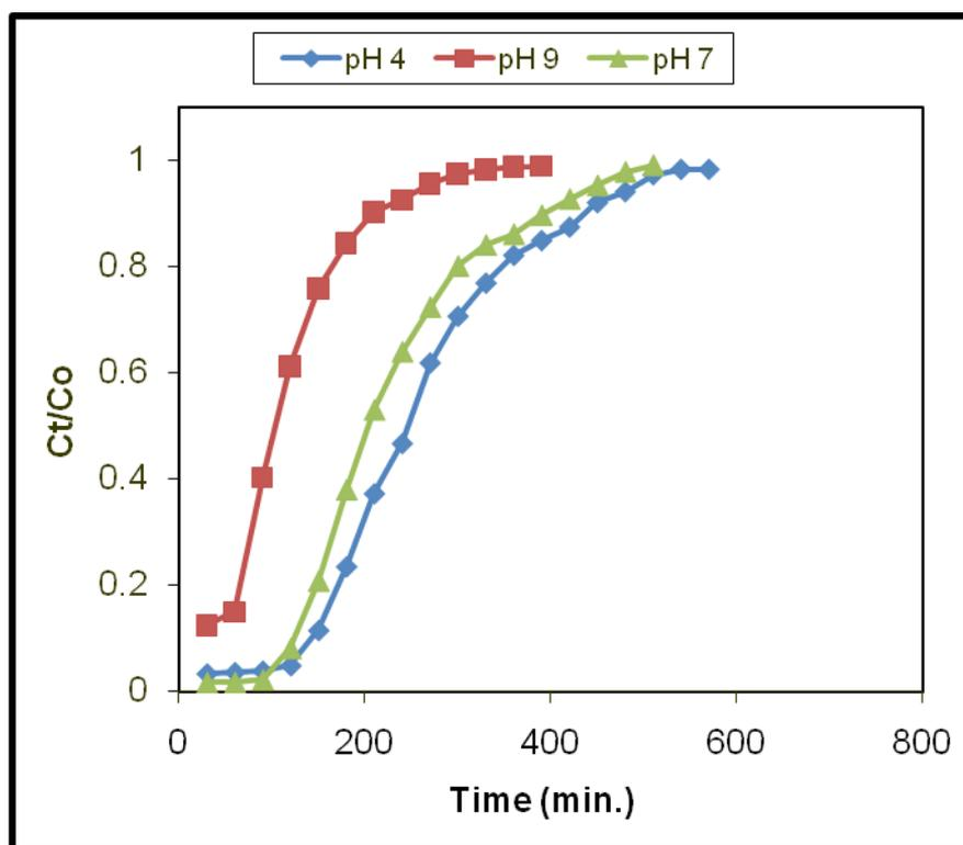
**Fig. 1. Breakthrough curves of the effects of pH values on biosorption of CR onto water hyacinth ( $F = 1 \text{ ml min}^{-1}$ ,  $C_o = 20 \text{ mg l}^{-1}$ )**
