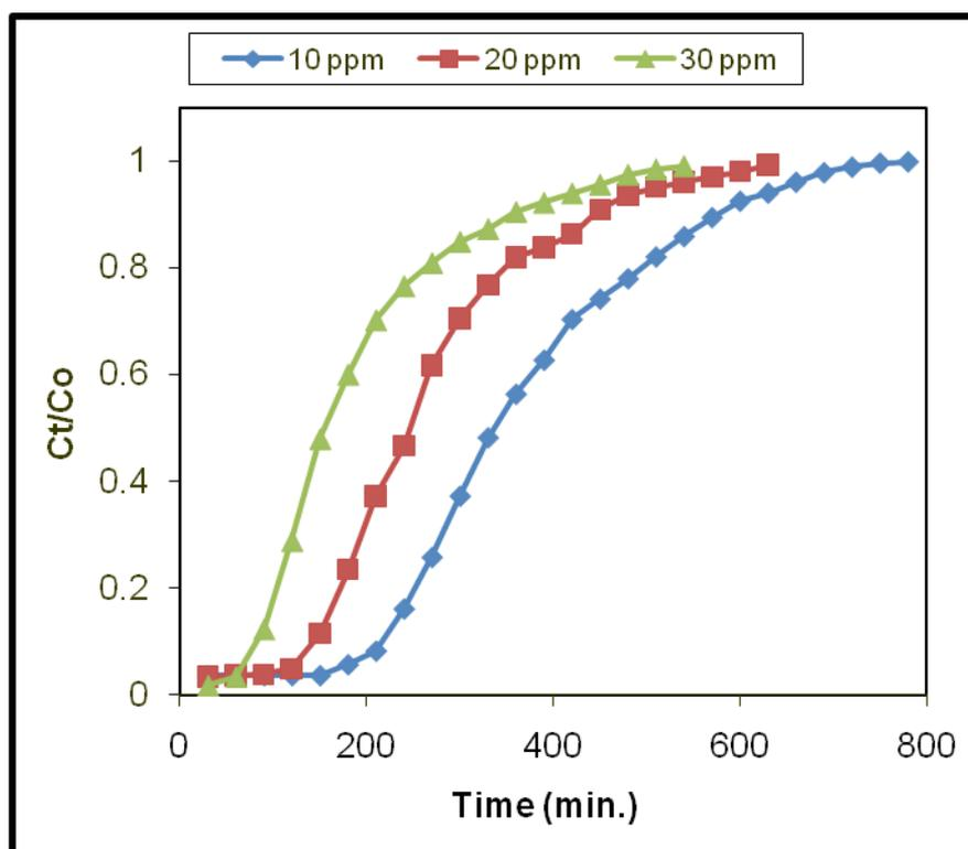
Fig. 4. Breakthrough curves of the effects of different conc. on biosorption of CR onto water hyacinth ( $F = 1 \text{ ml min}^{-1}$ ,  $C_0 = 20 \text{ mg l}^{-1}$ )
