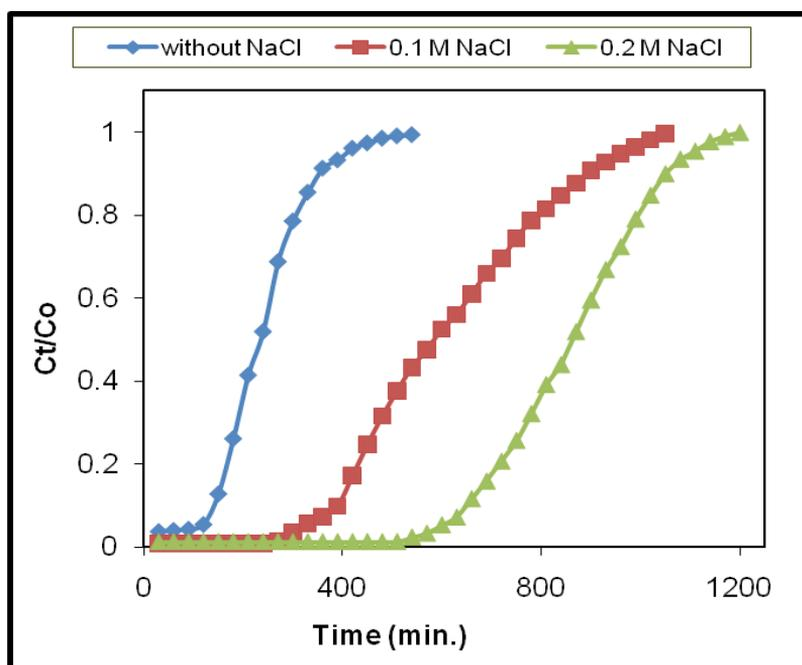
Fig. 5. Breakthrough curves of the effects of existing salt (NaCl) on biosorption of CR onto water hyacinth ( $F = 1 \text{ ml min}^{-1}$ ,  $C_o = 20 \text{ mg l}^{-1}$ )
