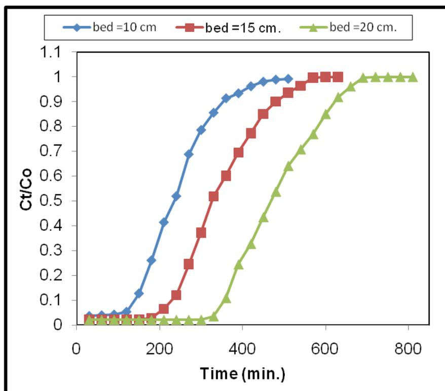
Fig. 3. Breakthrough curves of the effects of different bed depth on biosorption of CR onto water hyacinth ( $F = 1 \text{ ml min}^{-1}$ ,  $C_o = 20 \text{ mg l}^{-1}$ )
